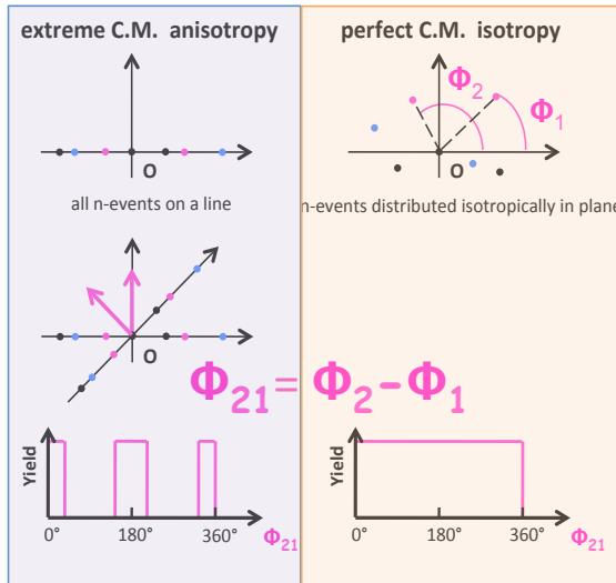
project fission axis and all n events on a plane  $\perp$  to fission axis
